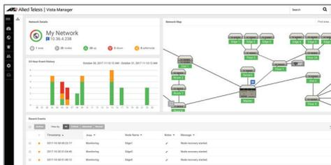
Critical issues, such as internal security threats, link tampering, network loops, environmental alarms, and failed nodes, are highlighted on the network map and in the event log so they can be easily dealt with. An integrated Syslog server shows informative messages from network nodes and alarms on the network map, while asset management enables firmware and configuration backup and upgrade of one, many, or all devices.
